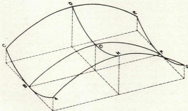
Fig. 3. Hyperbolic paraboloid limited by principal parabolas and considered as a translation surface.
