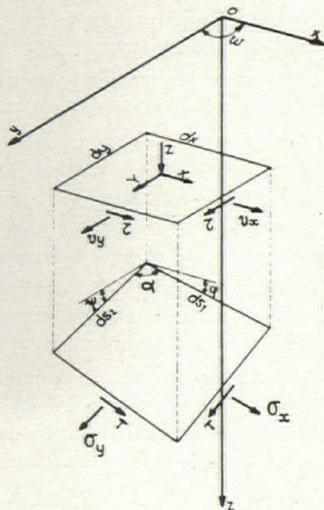
Fig. 2. External forces and internal forces which act on a surface element.
