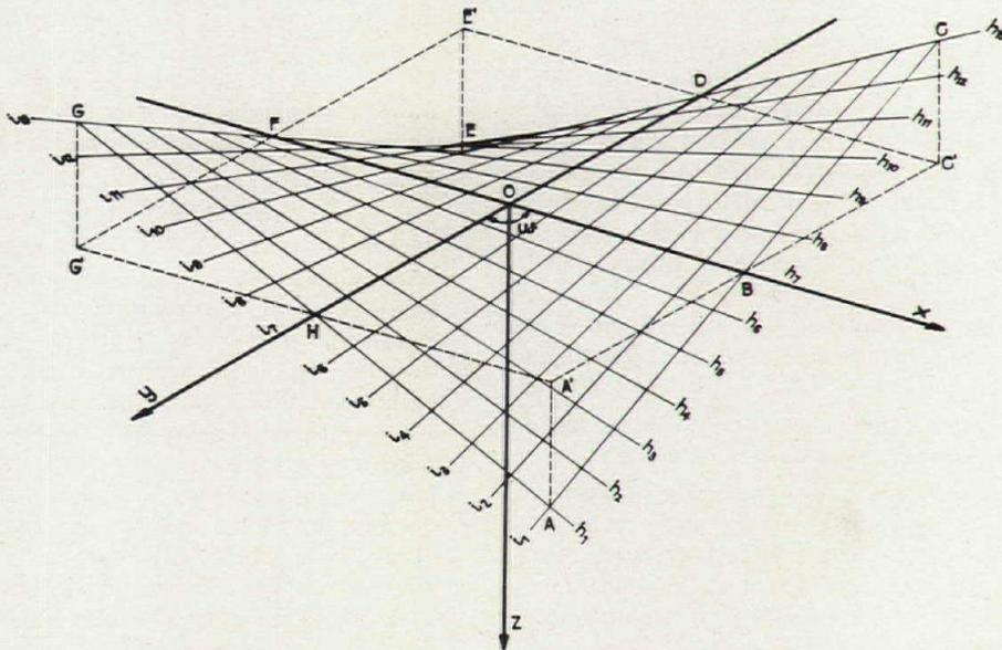
Fig. 1. Generation diagram of a hyperbolic paraboloid.
