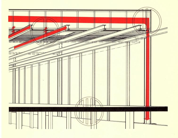
SPECIAL CONDITION: IMPORTANT CONNECTION, NOT STRUCTURALLY CONTINUOUS.
