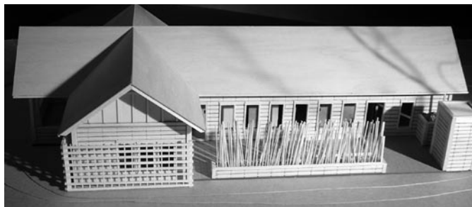
Features on this 1/4" scale model include rainwater catchment, bamboo privacy screen and architectural greenscreen. National jury commented on the simple elegance of the design scheme.
