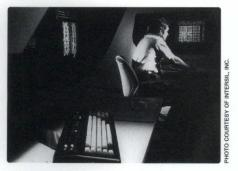
CALMA computer-aided design (CAD) workstation is used for integrated circuit design and gate array routing.
