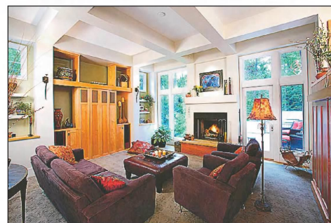
The beams in the living room ceiling were wrapped in dry-wall to help distinguish this area from adjacent zones.
