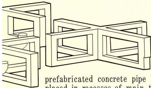
prefabricated concrete pipe hangers
