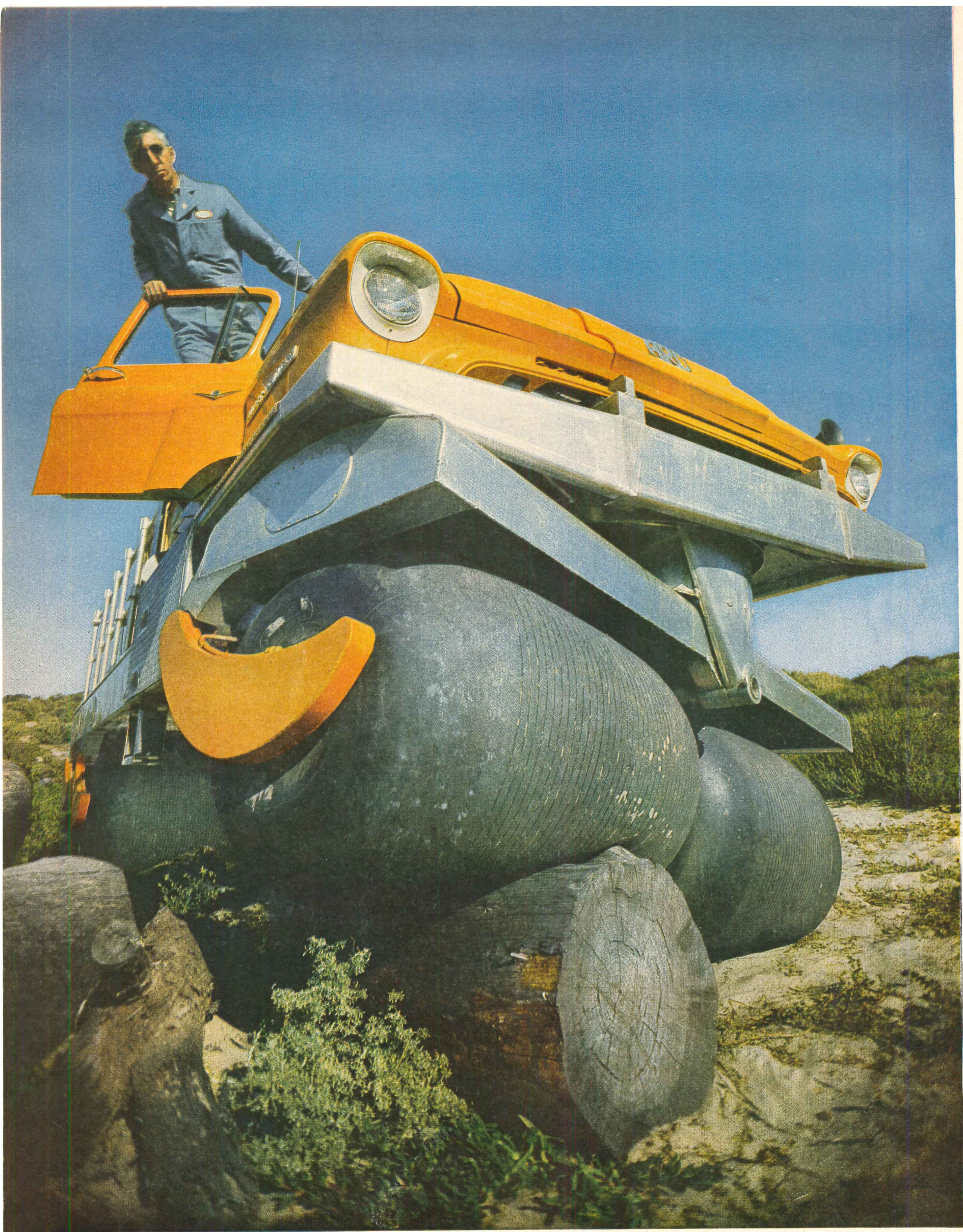
ROLLIGON , off-highway truck soon to be in regular production at Albee plant in Monterey, Calif., demonstrates how it can mush over heavy obstacles. The Rolligon has a seven-ton pay load and operates on six low-pressure (2-5 lb.)
