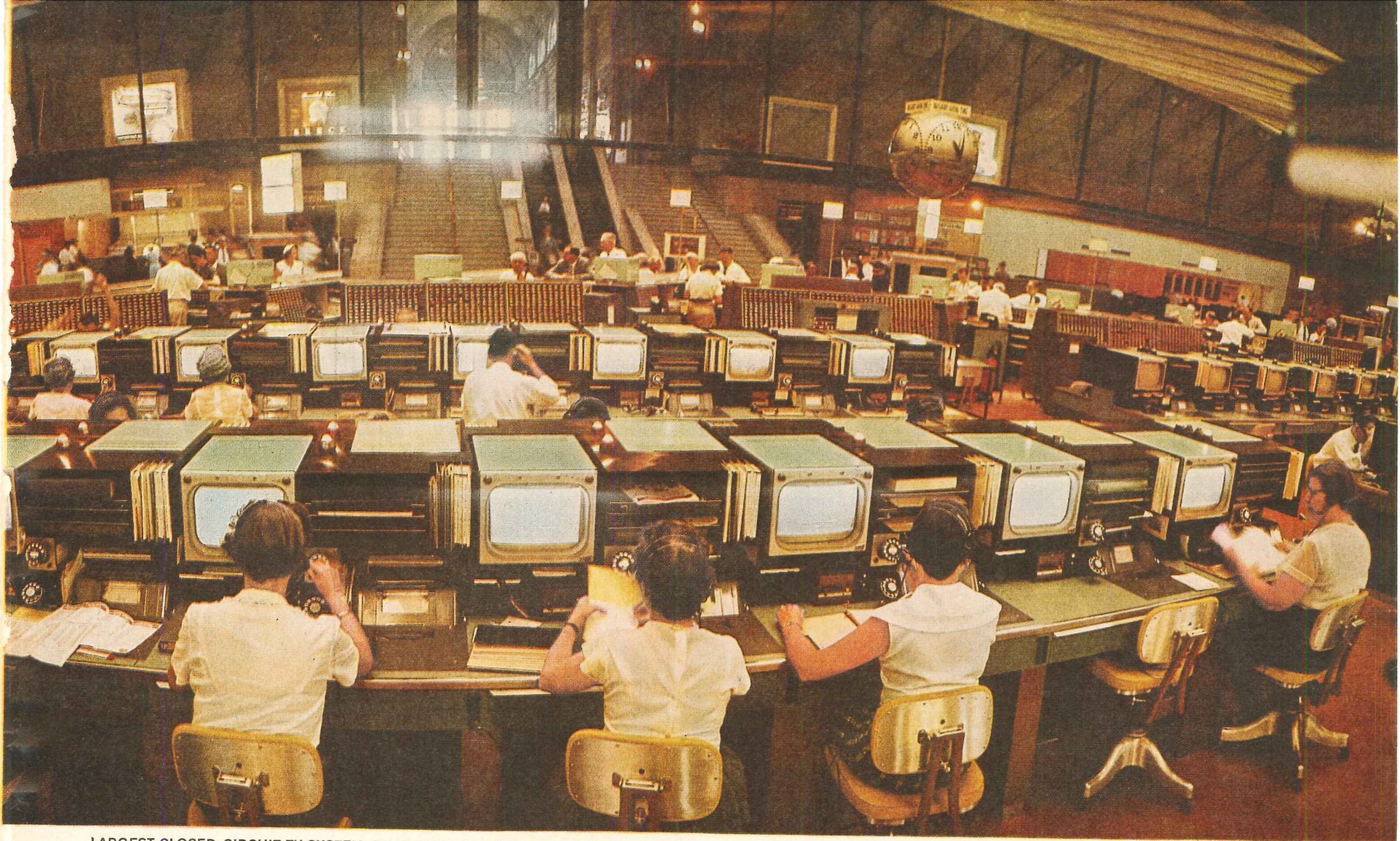
LARGEST CLOSED-CIRCUIT TV SYSTEM. BY DIALING CODE NUMBER, TICKET CLERKS AT COUNTER OR ON PHONES HAVE AVAILABLE TICKET SPACE FLASHED ON SET
