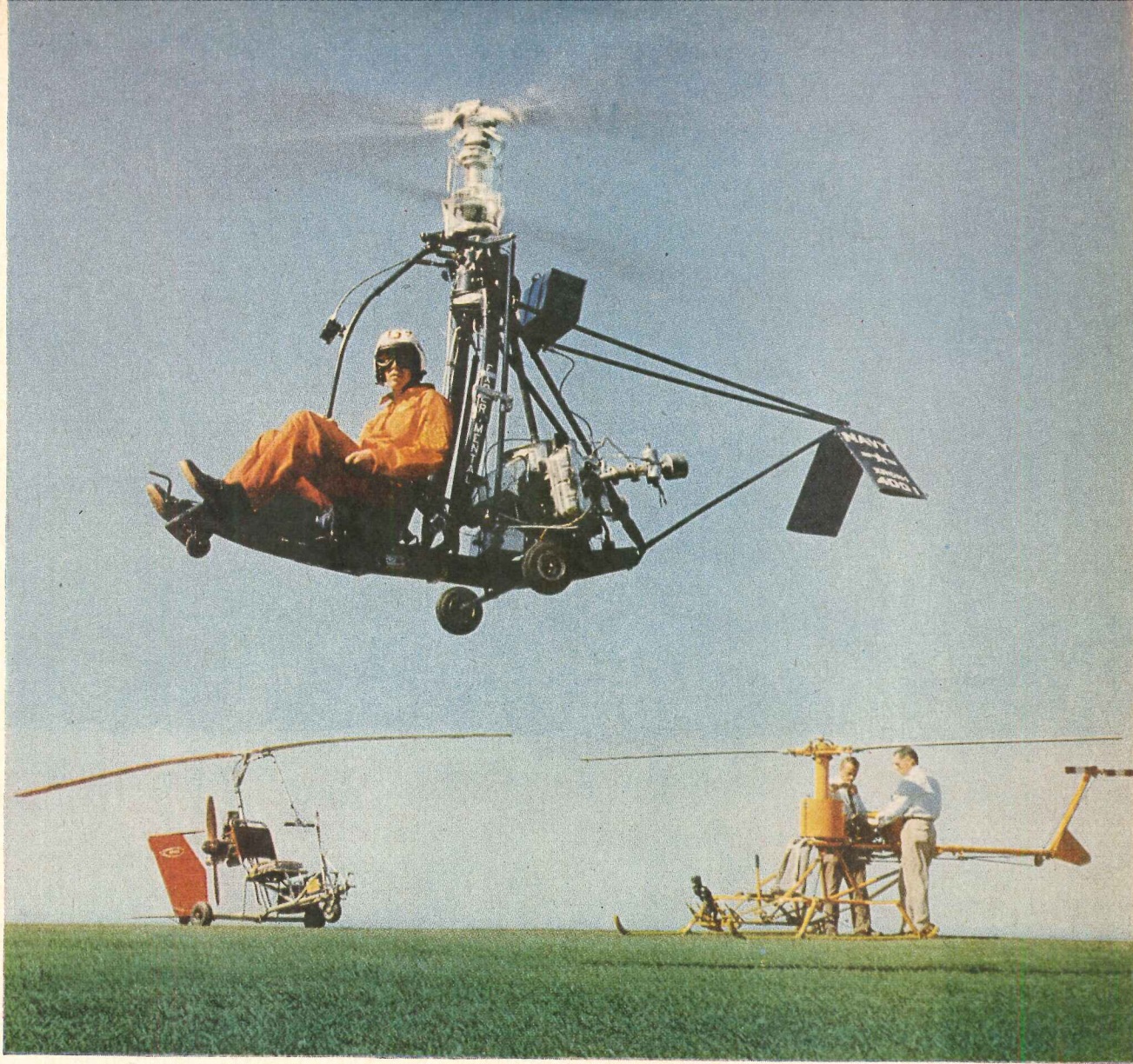
ONE-MAN AIRCRAFT in final stages of experiment are shown in three forms. At left is Bensen Gyro-copter, which does not hover, requires short
